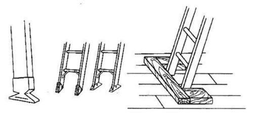
• All ladders must be equipped with safety (non-skid) feet.
