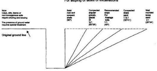
Approximate Angle of Repose For sloping of sides of excavations
