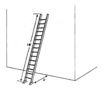
Portable ladders must be used at such a pitch that the horizontal distance from the top support to the foot of the ladder is about one-quarter of the working length of the ladder.
