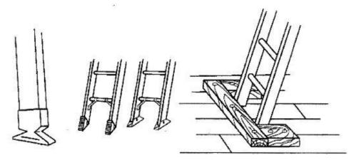
All ladders must be equipped with safety (non-skid) feet.
